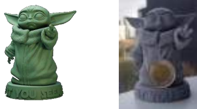
Figure. 2 A 3D model and the printed part – baby Yoda
