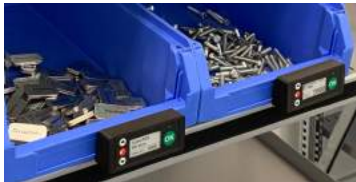
Figure. 19 Pick by light system for warehouses
