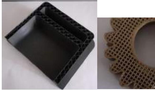
**Figure 14. The infill shape and density**
