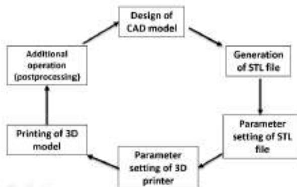
**Figure 3. Rapid prototyping cycle**
