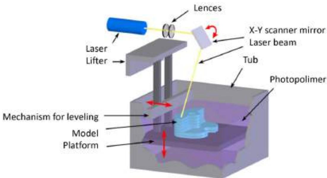
**Figure 21. Princip of SLA technology**
