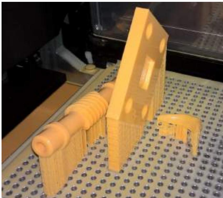
**Figure 23. Parts made by SLA technology directly after finishing printing**
