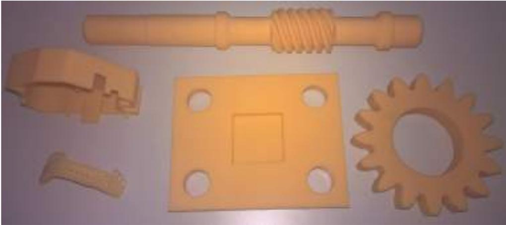
**Figure 22. Parts made by SLA technology**
