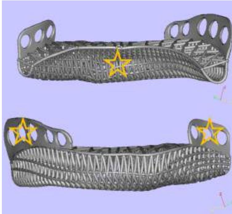
**Figure. 5 Position of support structure**
