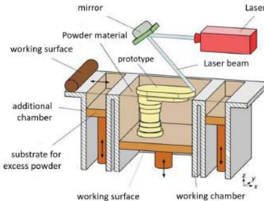
**Figure 27. Princip of SLS technology**
