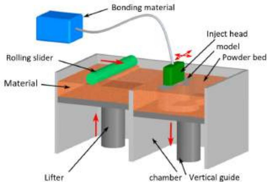
**Figure 28. Princip of BJ technology**
