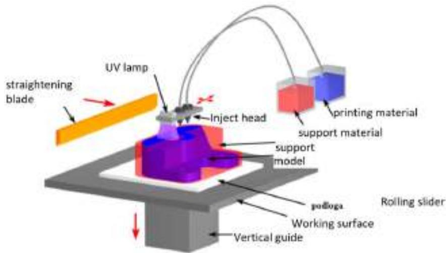
**Figure 29. Princip of Polyjet technology**
