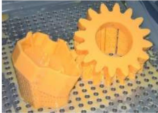
**Figure 24. Parts made by SLA technology directly after finishing printing**
