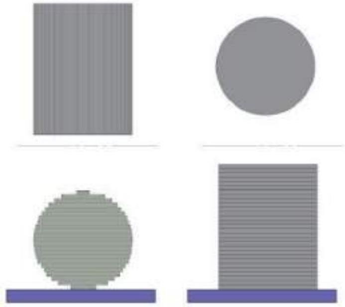
**Figure 26. Importance of positioning of part on the bed**
