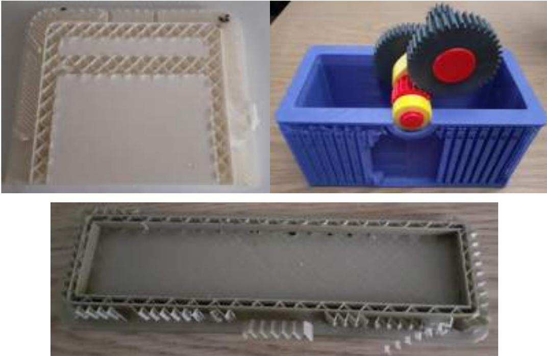
**Fig. 16. Different types for supports**
